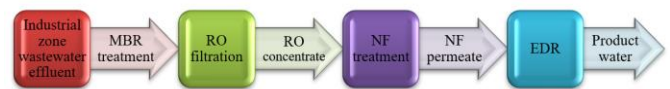
Fig. 1. Overall flow diagram of the integrated membrane process for concentrate management of RO process following MBR operation for wastewater treatment.
